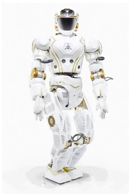
(iii) NASA JSC Robotics / Valkyrie - Building Gundams: Gundam Robotics Systems builds machines that remove the responsibility of humans to work in critical, yet hazardous environments. The NASA Robonaut Valkyrie was initially designed to remove humans from maintenance areas outside of the International Space Station.
